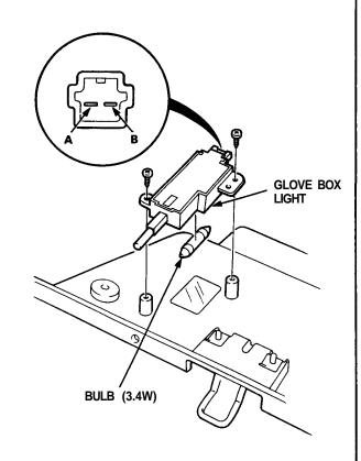
5. There should be continuity between the A terminal and B terminal with a bulb installed. There should be no continuity when the switch is pushed.
