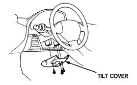
Remove the steering column lower cover and upper cover.
