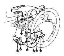
5. Disconnect the 16-P connector and 10-P connector.
