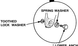
\* LOWER ANCHOR BOLT 7/16-20 UNF 32 N·m (3.2 kg-m, 23 lb-ft)
