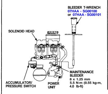
Connect the RED terminal from one solenoid to the battery positive (+) terminal with a remote starter switch. Connect the BLK terminal from the same solenoid to the battery negative (-) terminal with a jumper lead as shown.
