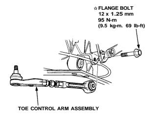
CAUTION: Make sure that the reference marks on the toe control arm are aligned.
