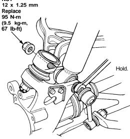
☆ Corrosion resistant bolt/nut
