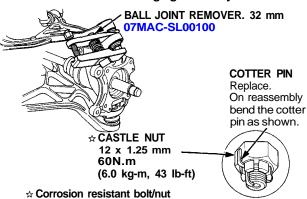
14. Separate the knuckle from the upper control arm and driveshaft outboard joint.
