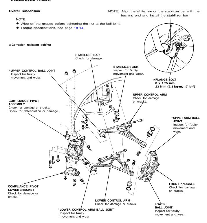
NOTE: Replace the joint boot if any are damaged. The parts marked with an asterisk (\*) have a retainer attaching the ball joints. Replace the retainer whenever the boot is replaced.
