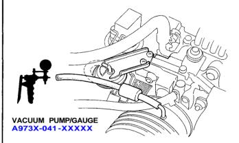
3. Apply vacuum and check the speed the vacuum goes out.
