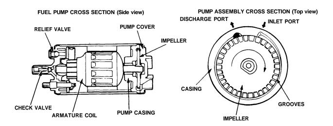
The fuel pump is comprised of a DC motor, a circumference flow pump, a relief valve for protecting the fuel line systems, a check valve for retaining residual pressure, an inlet port, and a discharge port. The pump assembly consists of the impeller (driven by the motor), the pump casing (which forms the pumping chamber), and the pump cover.
