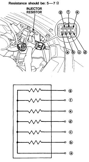
• Replace the resistor with a new one if any of the resistances are outside of the specification.
