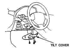
Remove the steering column lower cover and upper cover.
