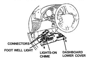
Disconnect the 18-P connector from the floor wire harness.
