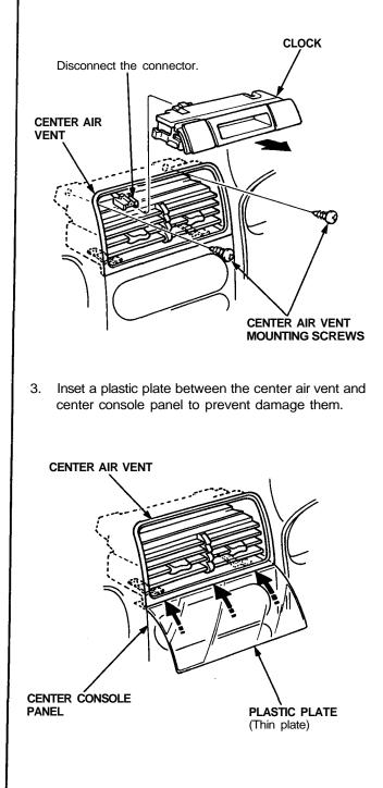
4. To make a gap between the center air vent and dashboard, pull the top of the center air vent while lowering it as shown.
