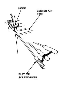
8. Pull the center air vent backward while prying the hook.
