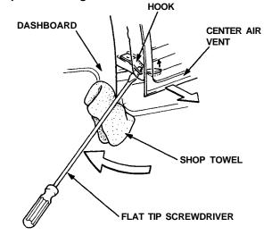
9. Detach the another hook as the same work, then remove the center air vent.
