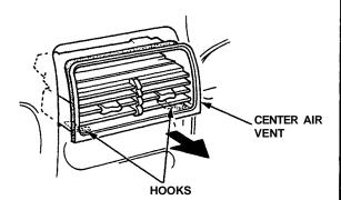
10. Install the center air vent and clock.
