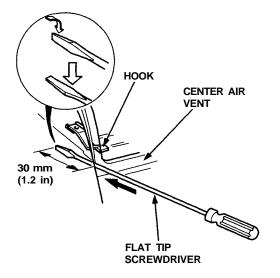
Inset the tip of a flat tip screwdriver in under the hook by turning a flat tip screwdriver. Detach the hook by prying it.
