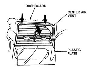
5. Inset a flat tip screwdriver between the center air vent and dashboard as shown.
