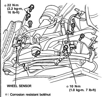
6. Remove the banjo bolt and disconnect the brake hose, then remove the brake hose clamp from the knuckle.
