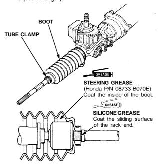
Install the new boot bands on the boot and bend both sets of locking tabs.
