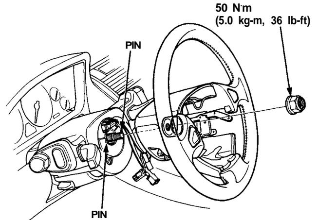
3. Insert the cruise control set/resume 4-P connector and airbag 3-P connector to the steering wheel clips.
