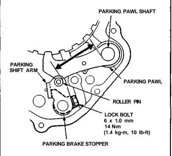
7. Install the special tool as shown, and shift to P position.
