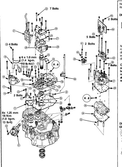
NOTE: Install the oil pump driven gear with its chamfered side facing down.
