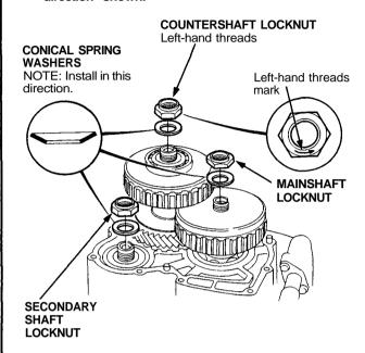
9. Tighten the locknuts to specified torque.
