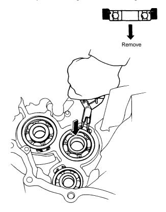
2. Expand each snap ring with the snap ring pliers, insert the new bearing part-way into it, then release the pliers. Push the bearing down into the transmission until the ring snaps in place around it.
