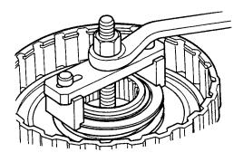
8. Install the circlip.
