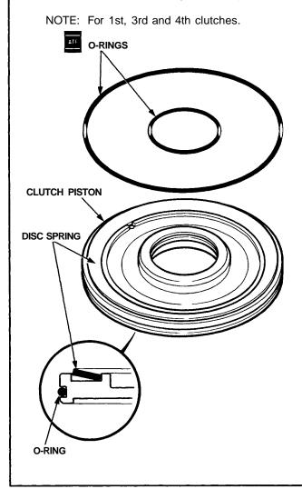
4. Install the piston in the clutch drum. Apply pressure and rotate to ensure proper seating.
