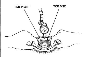
15. If the clearance is not within the service limits, select a new clutch end plate from the following table.
