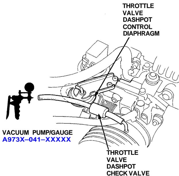
3. Apply vacuum and check the speed the vacuum goes out.
