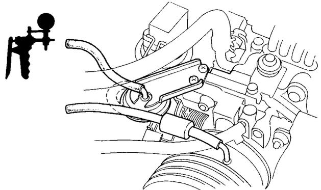
5. Apply vacuum and check that the rod pulls in and vacuum holds.
