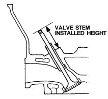
If valve stem installed height is over the service limit, replace valve and recheck. If still over the service limit, replace cylinder head; the valve seat in the head is too deep.
