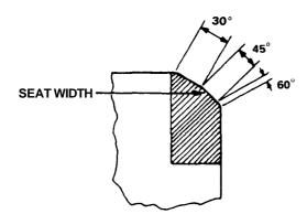
After resurfacing the seat, inspect for even valve seating: Apply Prussian Blue compound to the valve face, and insert valve in original location in the head, then lift it and snap it closed against the seat several times.
