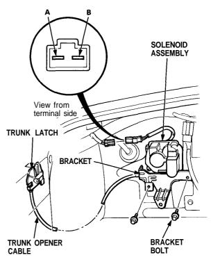
3. To remove the solenoid, remove the two bolts, then disconnect the trunk opener cable from the solenoid assembly.
