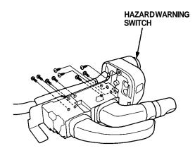
8. If necessary, remove the hazard warning switch bulb.
