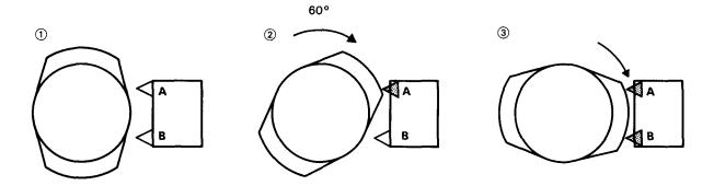
The cancel unit monitors the on-off sequence of both switches. Once it receives a full set of signals for a right or left turn, it energizes the solenoid which then moves the turn signal lever back to neutral.
