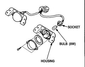
3. If necessary, separate the lens from the housing by removing the two screws.
