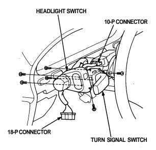
If necessary, remove the turn signal cancel unit and cancel switch.
