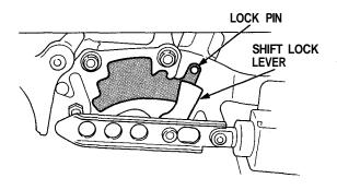
If it is not blocked, adjust the position of the shift lock solenoid as needed to block it.
