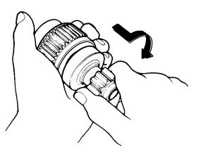
Check if the starter drive gear is worn or damaged. If the gear is worn or damaged, replace the overrunning clutch assembly; the gear is not available separately.
