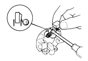
2. Install the armature in the housing. Next pry back each brush spring again, and push the brush down until it seats against the commutator. Then release the spring against the end of the brush.
