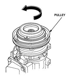
• Measure the clearance between the pulley and the pressure plate all the way around. If the clearance is not within specified limits, the pressure plate must be removed and shims added or removed as required, following the procedure on page 22-40.
