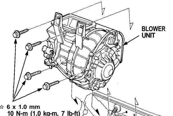
6. Install the blower unit in the reverse order of removal, then make sure it runs and doesn't leak any air.
