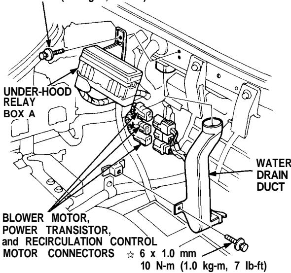
5. Remove the mounting bolts, then remove the blower unit.
