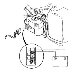
Plug the connector back into the motor. Operate the mode switch on the climate control unit to each mode. Verify that the mode control motor has moved to the selected position by checking the air flow for the mode selected.
