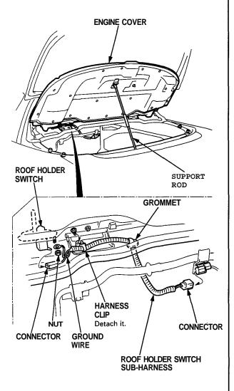
Remove the support rod from the engine cover. Remove the bolts, than remove the engine cover.
