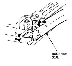
Install the side portion of the roof side seal into the roof side retainer as shown.
