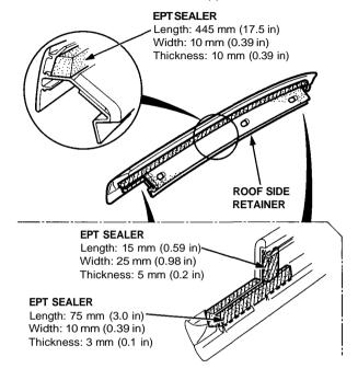
10. If the old roof side seal is to be reinstalled, scrape the old butyl tape from each end of it, then clean each end with alcohol. Glue the new butyl tape on each end as shown.
