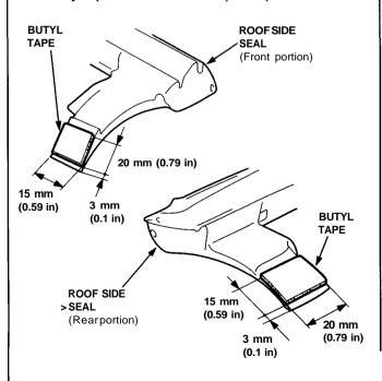
11. Install the roof side retainer.
