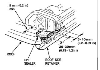
14. Engage the lip of the roof side seal with the groove of the roof side retainer as shown, then gently set each end of the roof side seal down on the sealant.
