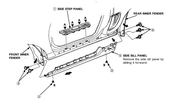
To install the side sill panel, remove the clips from the body, install them on the panel, then install the panel on the car.
