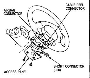
Connect the special tool to the cable reel connector.
