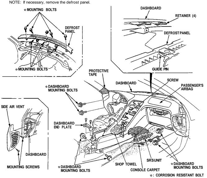
8. Installation is the reverse of the removal procedure.
