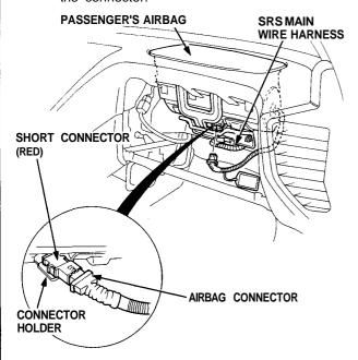
Connect the special tool to the SRS main wire harness connector.
