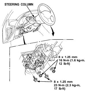
3. Remove the nuts, then remove the airbag bracket (passenger's).
