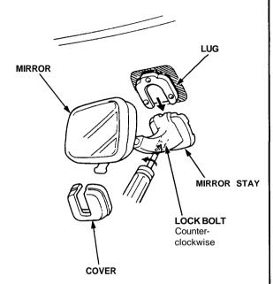
3. Remove the lock bolt, then remove the toothed lock washer and hold spring from the mirror stay.
