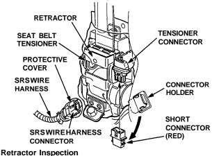
CAUTION: When checking the retractor, do not touch the seat belt tensioner.
