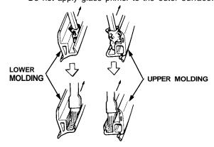
Run a bead of adhesive in the upper and lower molding grooves.
