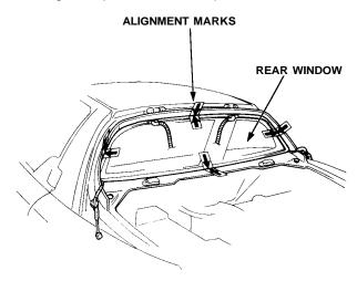
12. Glue the upper and lower rubber dams to the inside face of the rear window, as shown, to contain the adhesive during installation.
