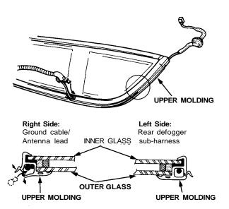
11. Set the rear window upright on the body, then center it in the opening. Make alignment marks by marking lines across the rear window and body with a grease pencil at the four points shown.
