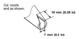
17. Pack adhesive into the cartridge without air pockets to ensure continuous delivery. Put the cartridge in a calking gun, and run a bead of adhesive around the edge of the rear window as shown.
