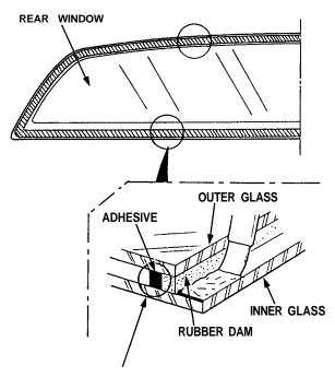
NOTE: Be careful not to cut the adhesive and rubber dam between the inner glass and outer glass. 4. Clean the rear window surface with alcohol where the new moldings are to be installed.
