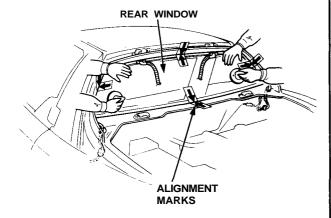
After the adhesive is dry, spray water over the rear window and check for leaks. Mark leaking areas and let the rear window dry, then seal with sealant.
