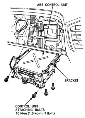
6. Installation is the reverse of removal procedure.
