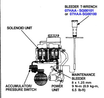
5. Connect the RED terminal from one solenoid connector to the battery positive (+) terminal with a remote starter switch. Connect the BLK terminal from the same solenoid to the battery negative (-) terminal with a jumper lead as shown.
