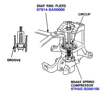
15. Install the adjusting nut, adjusting spring A, and washer, then secure with the circlip.
