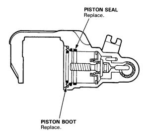
17. Coat the outside of the piston with silicone grease, and install it on the adjusting bolt while rotating it clockwise.
