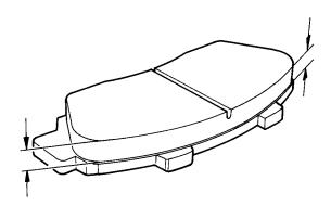
NOTE: Measurement does not include pad backing thickness.
