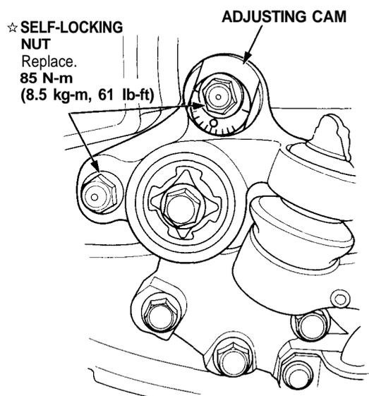
☆: Corrosion resistant bolt/nut
