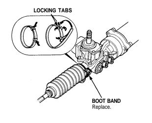
9. If the tie-rod ends were removed, install the tie-rods on the right and left rack ends and screw them in until the threaded section is 11 mm (0.4 in) in length.
