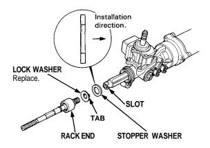
6. Tighten the rack end securely, then bend the lock washer back against the flat on the flange as shown.
