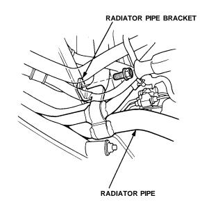
17. Remove the radiator pipe bracket at the floor, and space the radiator pipe away from and gearbox.
