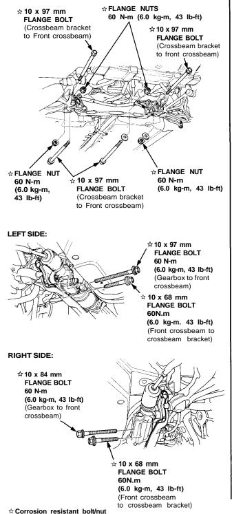
Lower the gearbox and front crossbeam with care so as not to interfere with the radiator pipe.
