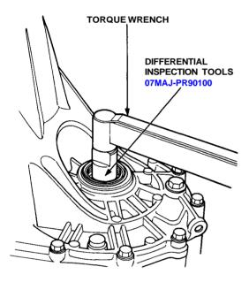
7. If the bearing preload is not within the standard, select the shim that will give you the correct preload, and recheck.
