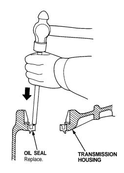
3. Remove the oil seal from the torque converter housing.
