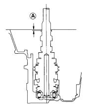
Set the mainshaft ball bearing in the clutch housing, and measure distance
