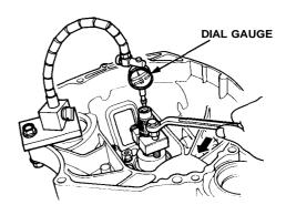
f. Turn the mainshaft holder bolt clockwise; stop turning when the dial gauge has reached its maximum movement. The reading on dial gauge is the amount of mainshaft end play.
