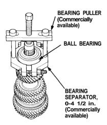
4. Remove the bearing outer race from the needle bearing, then remove the needle bearing using a bearing puller as shown.
