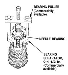
CAUTION: Remove the gears using a press and steel blocks as shown. Use of a jaw-type puller can damage the gear teeth.
