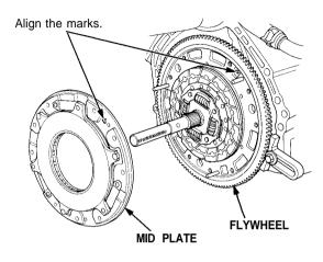
5. Install the 1st clutch disc.
