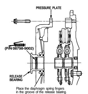
8. Torque the mounting bolts in a crisscross pattern as shown. Tighten them several steps to prevent warping the diaphragm spring.
