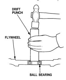
3. Drive the new ball bearing into the flywheel using the special tools as shown.
