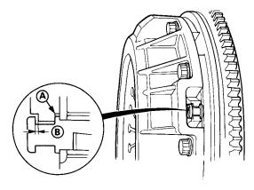
4. Initialize the remaining mid plate guides as described above, then remove the 5 mm bolt.
